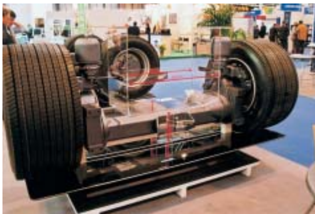
Arvin Meritor showed this portal axle for low-floor buses. By using super single wheels and tyres, there is not only a saving in weight, but also increased width in the gangway, between the wheels
