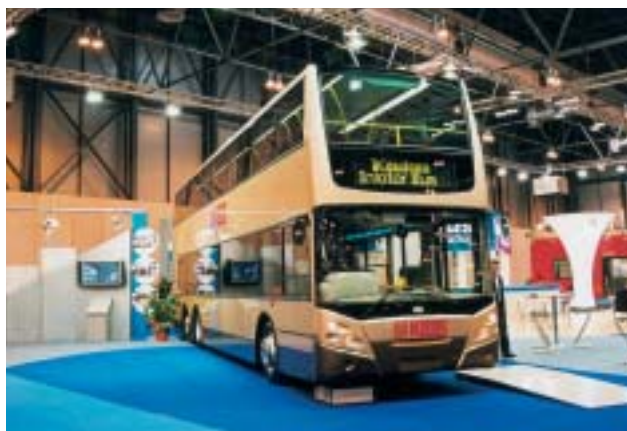
TransBus International showed this 12 metre air conditioned double decker for Kowloon Motor Bus of Hong Kong. The use of a ZF 6-speed fully automatic gearbox has achieved considerable savings in fuel economy
