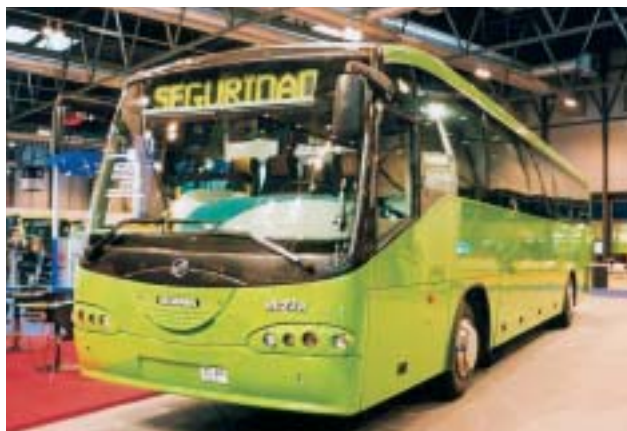
A 12,8 metre inter-urban coach by Irizar, the largest bodybuilder in Spain mounted on a Scania chassis
