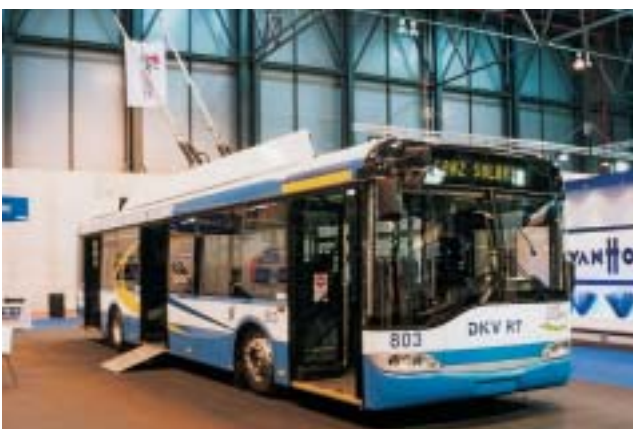
Solaris of Poland built this low-floor trolley-bus for the Hungarian city of Debrecen. Ganz Transelektro of Budapest supplied the electrical equipment
