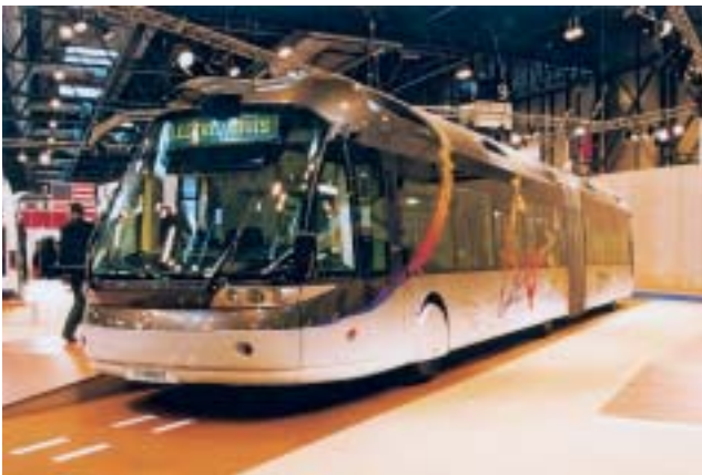
It was a surprise to find three trolley-buses in the exhibition. This was an articulated version of the Irisbus CIVIS, complete with its optical guidance system
