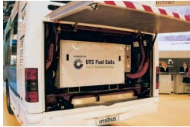
The compact United Technologies Company fuel cell in the rear of the Irisbus vehicle
